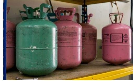
N. The ODS & HFC Reserve accepts burned out or mixed reserve products. Mixed cylinders are categorized by the predominate gas, which needs to be a gas managed by the ODS & HFC Reserve. All contents need to be clearly identified with all chemical components (i.e., R236fa & R134a). If cylinders contain gases that are not managed by the ODS & HFC Reserve, they need to be disposed of by other means.
